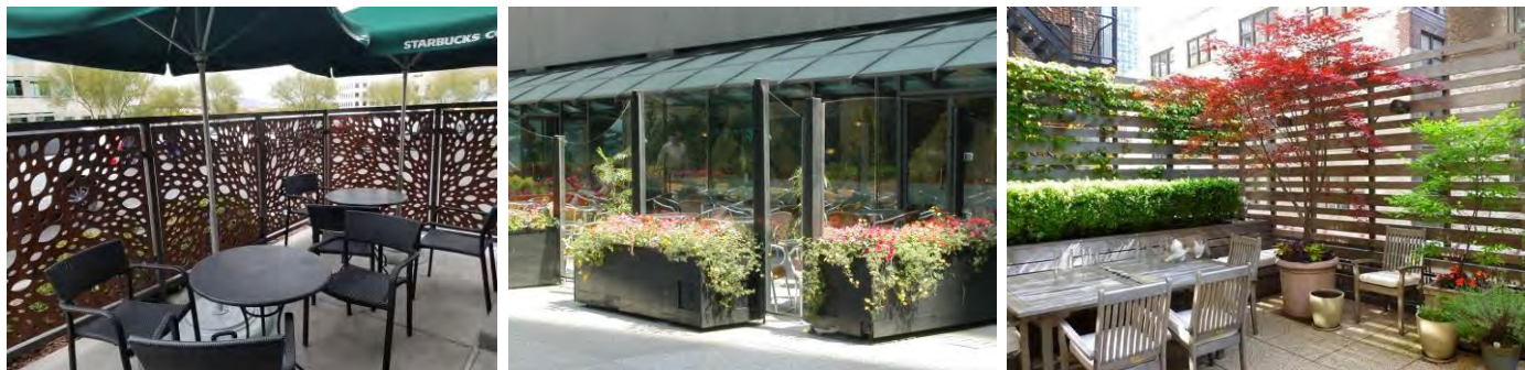
Image 12: Design strategies for wind control for ground level outdoor amenities
